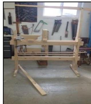
The second workshop allowed for practice on the completed lathe and the start of the next project: the flax brake. One final piece has been added to the lathe: a small board to direct the drive belt and control its lateral movement along turning.
